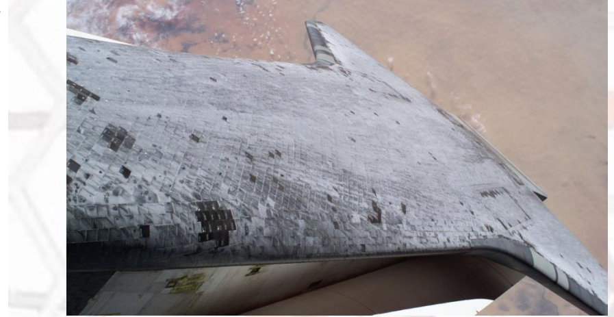
STS-114 Discovery thermal protection system (S114-E-6412)
