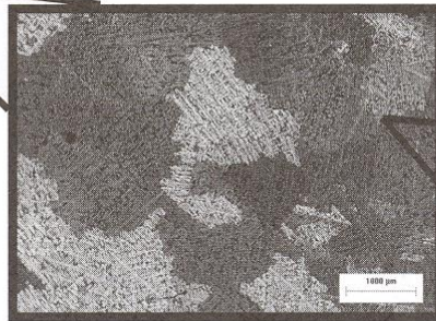
Microstructure - Grains ≅ 1 – 10 millimeters
