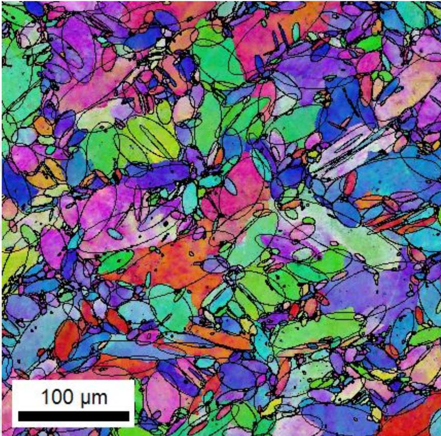
Ellipses can be fitted to each grain
