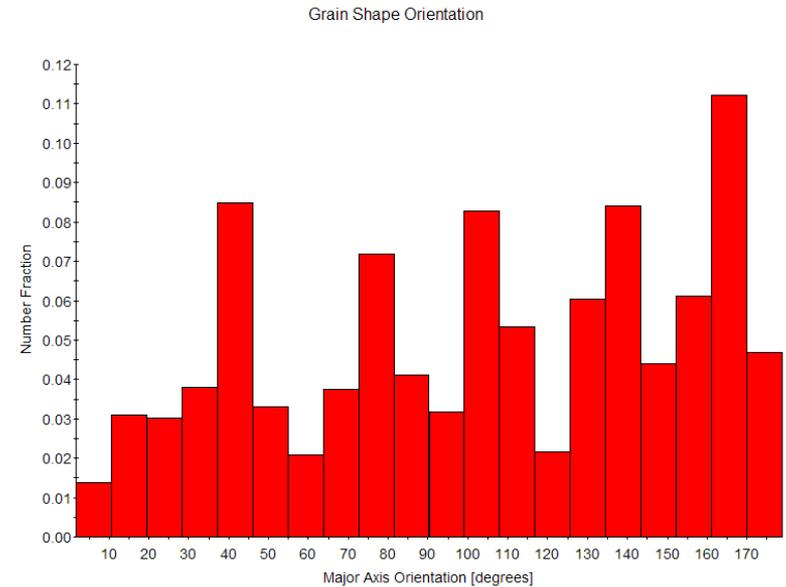
Here the direction of the major axis of each ellipse is plotted relative to the horizontal direction
