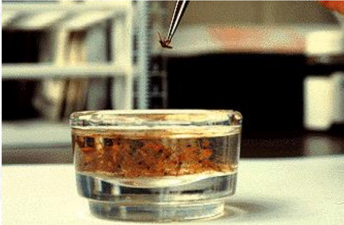
**Samples have to be prepared carefully to withstand the vacuum inside the microscope.**
