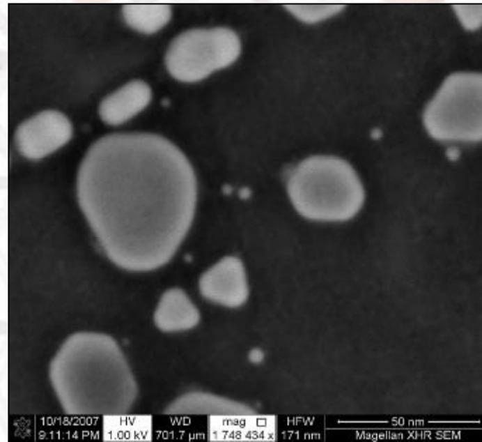
Gold particles on carbon test sample, imaged at 15kV (left, HFW of 300nm) and 1kV (right, HFW of 171nm).
