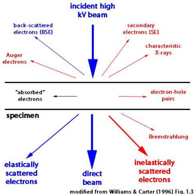
1. SEM gives ***images of the microstructure*** of a specimen with the resolution  $\sim 1\text{ nm}$ ; the range of the acceleration voltage  $50\text{ eV} - 30\text{ kV}$ .
