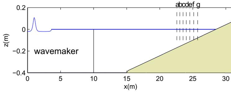
Fig. 1. Experimental setup for regular wave breaking test. Gauges (a–g) are at still water depths [0.169, 0.156, 0.142, 0.128, 0.113, 0.096, 0.079] m, respectively.
