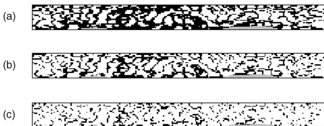
Fig. 6. The number of fragile bits depends on the threshold used. There are fewer bits that flip in at least 40 percent of the iris codes than there are that flip in at least 20 percent of the iris codes. (a) p = 20\% . (b) p = 30\% . (c) p = 40\% .
