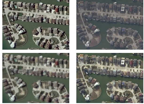
Figure 2. (Top left) Source image. (Top right) Target image. (Bottom left) 11X11 windows, artifacts visible. (Bottom right) 101X101 windows, no artifacts visible.
