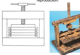
Figure 11. Representation of the oil press and modern reproduction.
