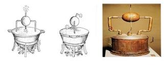
Figure 14. Representations of the steam boiler from Heron's writings and physical reconstruction of the device.
