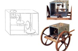
Figure 15. Heron's odometer and reconstructions of the odometer by Woodcraft.
