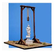
Figure 12. The monokolos hoisting machine.
