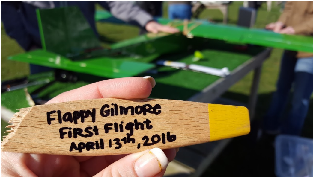
Figure 16. Propeller Damage after First Flight
