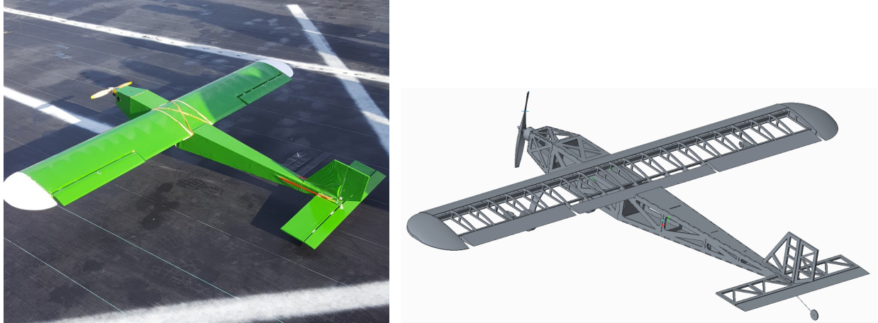
Figure 14. Final Build vs. Final CAD Model
