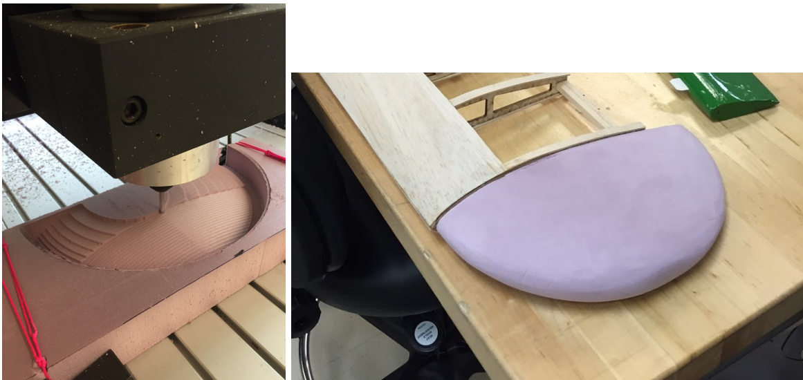
Figure 11. Wing tip milling and final model.
