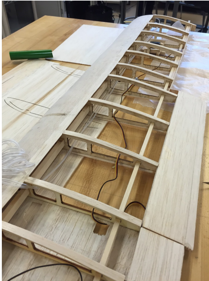
Figure 9: Wing construction, with balsa sheets on the leading edge and the wing ribs.
