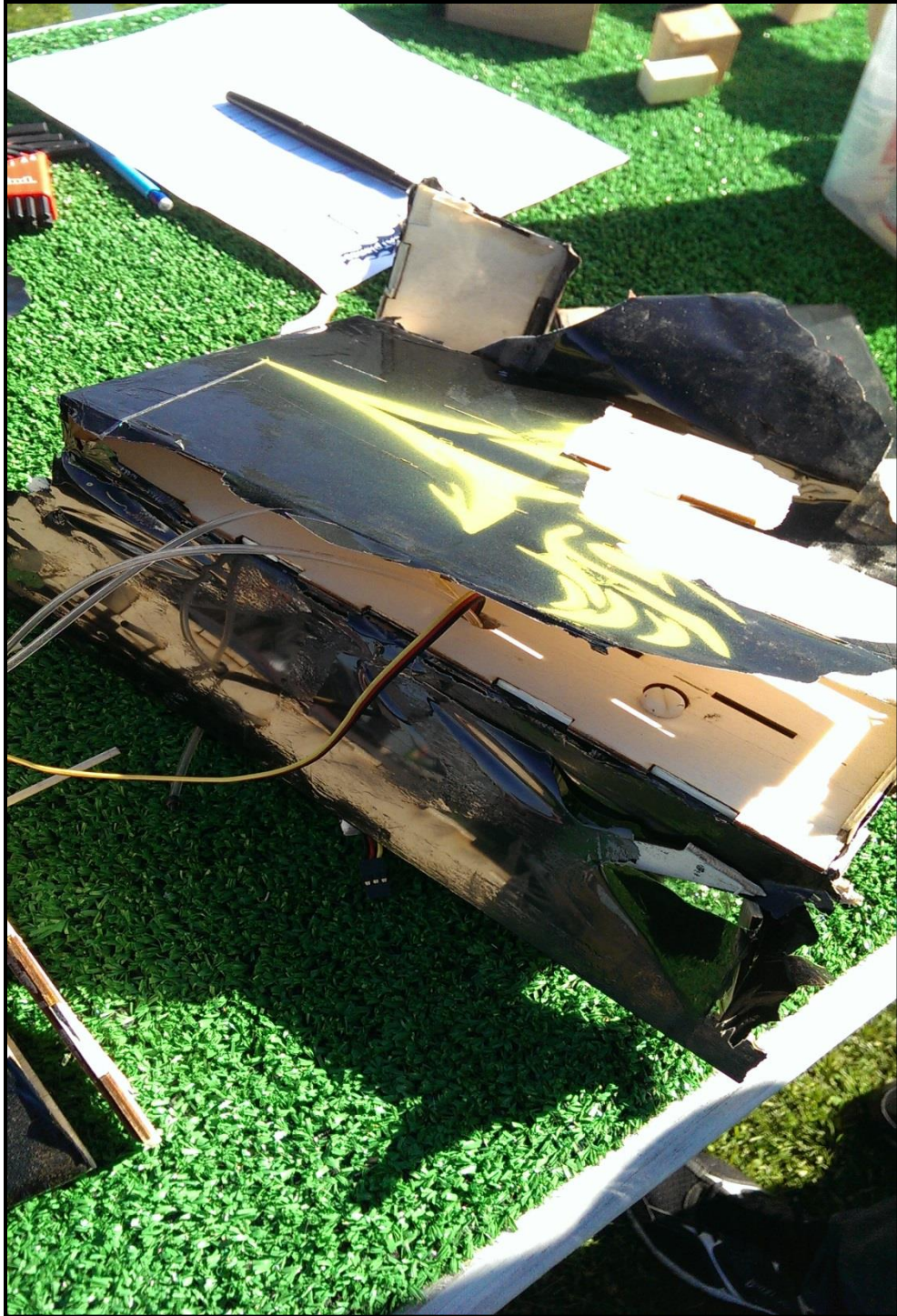
Figure 20. Wingbox after the crash.
