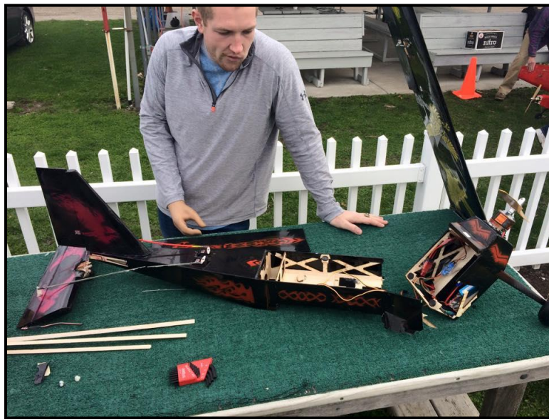
Figure 10. Photographic evidence of the damage our plane sustained from the harsh landing.
