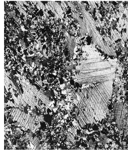
Partial replacement of CW grains: 4s 580 C
