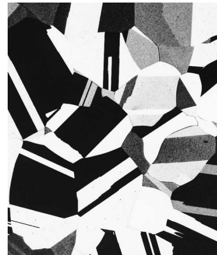
Partial replacement of CW grains: 4s 580 C
