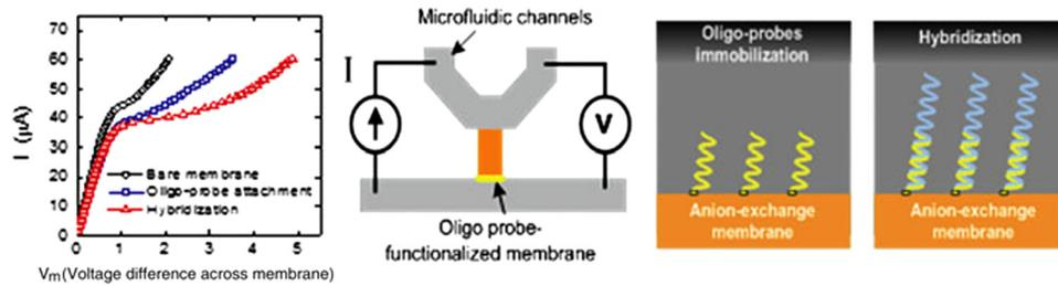
FIG. 9. Nonlinear PNP and PN membrane sensors for cytokine and mRNA. Molecular docking produces a surface membrane with an opposite charge. This nonlinear ion dynamics due to molecule docking produces hysteretic IV with nonlinear amplification of the ion current signal for the docking events. (Note that the signal is on the order of several volts instead of the usual mV in electrochemical sensing.) These membrane components can be integrated into the culture scaffold in Fig. 1.
