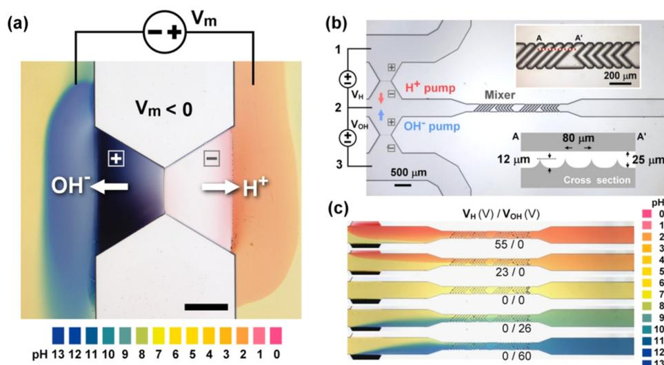
FIG. 7. An on-chip bipolar membrane  $p\text{H}$  actuator. The image in (a) shows how a DC field across a bipolar membrane can dissociate water and generate protons and hydroxyl ions at a controllable rate. Two such bipolar membranes are fabricated up stream of a flow channel and the protons/hydroxyl ions are mixed by a static mixer into a buffer of a specific  $p\text{H}$  between 2 and 10 in (b). The mixed streams are shown in (c) with a color chart for the universal  $p\text{H}$  dye.
