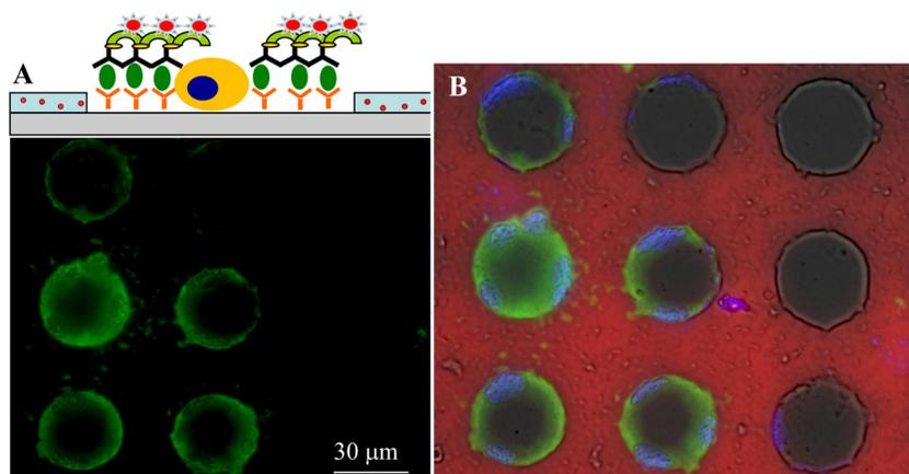
FIG. 6. Merged brightfield/fluorescence image showing integration of hydrogel-based  $\text{H}_2\text{O}_2$  sensor with TNF sensor. (a) Macrophages were treated with LPS for 3 h and the sample was stained with biotinylated anti-TNF Ab and neutravidin-FITC. The green fluorescence indicates secreted TNF from cells. (b) The addition of  $1 \mu\text{M}$  of  $\text{H}_2\text{O}_2$  and Amplex Red resulted in appearance of red fluorescence signal in the PEG hydrogel walls.
