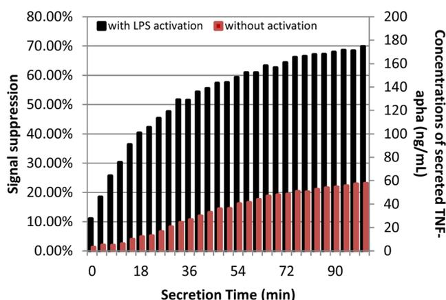
FIG. 5. Continuous monitoring of TNF from monocytes captured and cultured next to sensing electrodes analogous to those described in Figure 4. Measurements are taken every 4 min. Signal suppression—decrease in signal due to binding of cytokine molecules—is correlated to TNF concentration through calibration curve (not shown).
