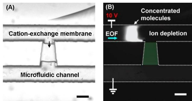
FIG. 8. (a) Optical microscopic image of a charge-selective membrane based preconcentrator. (b) Concentration of fluorescently labeled molecules taking place 10 s after applying a voltage bias of 10 V. The scale bars represent 50  $\mu\text{m}$ .
