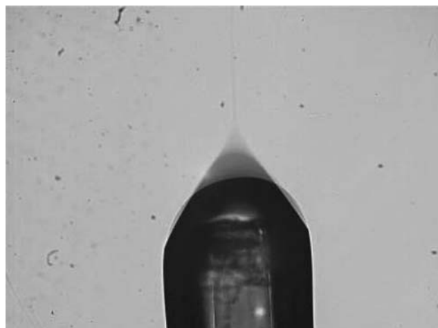
Fig. 8 An image of the stable Taylor cone and nano-fluidic jet of the electro-spray. Fluid EDTA-Tris; potential 3.5 kV; capillary: i.d. 100 \mu\text{m} , o.d. 365 \mu\text{m}
