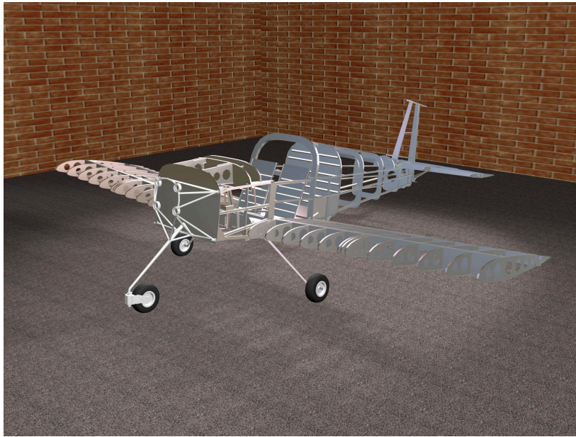
CAD of the internal structure of the aircraft (by A. Scott-Murphy – Honours student, 1997)
