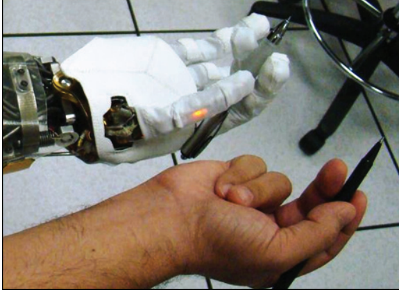
Fig. 2. The R2 hand and fingers approximate the size of a human hand.
