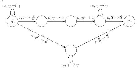
(d) Cycle through the queue and move the # right by one position. That is, pull symbols and push them back until we pull #; pull one symbol and push it; push #; continue pulling and pushing until \$ is reached. To handle the right end of the tape, if \$ immediately follows the new position of #, insert a blank.
