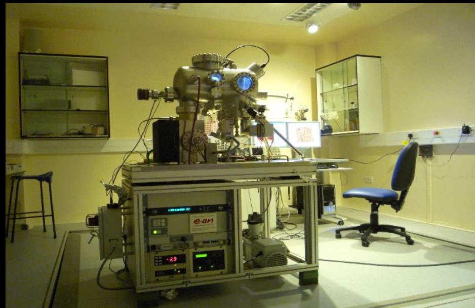
NSQI- Ultra-quiet Laboratory UHV SPM with Radiative heating
