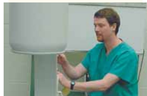
James J. Mason, associate professor of aerospace and mechanical engineering, adjusts the fluoroscope during cadaver tests to better monitor the location of the thermocouples and changes to the bone cement during the curing process.
