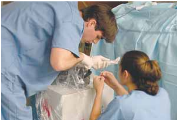
Working with researchers from Zimmer, Inc., Notre Dame undergraduates Peter Mack and Rebecca Brownlee prepare to monitor the temperature distribution of bone cement on a cadaver during the cement curing process. The device they are testing is the new hip fracture implant developed as a result of the collaboration between Notre Dame and Zimmer.
