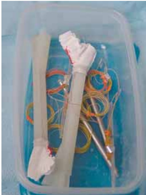
Peter Mack and Rebecca Brownlee, students in the Department of Aerospace and Mechanical Engineering, developed the procedure and apparatus, shown here, through which temperatures during the bone cement curing process could be measured in a cadaver model.
