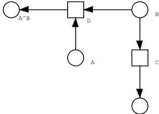
Fig. 2. Inhibiting transition D between place A and B.
