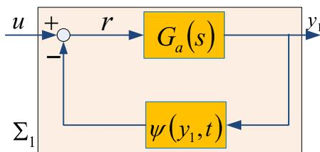
Fig. 7. Feedback connection
