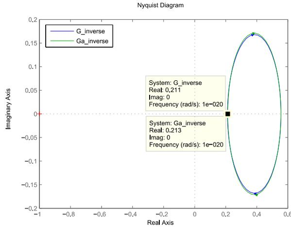
Fig. 6. The Nyquist Plots of  $G^{-1}$  and of  $G_a^{-1}$  in Example 2.
