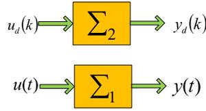
Fig. 3. Sampled-data System with an ideal sampler and a ZOH device, for which  $u(t) = u_d(k)$  for  $kh \leq t < (k+1)h$ ,  $y_d(k) = y(kh)$  for all  $k \geq 0$ , where  $h$  represents the sampling period.
