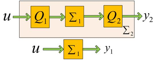
Fig. 4. Quantized-input, Quantized-output system:  $\Sigma_1$  satisfies (27) and the quantizer  $Q_i$  satisfies (26) with  $a_i u^T u \leq u^T Q_i(u) \leq b_i u^T u$ . The control input  $u$  and the outputs  $y_1, y_2$  are of the same dimensions.
