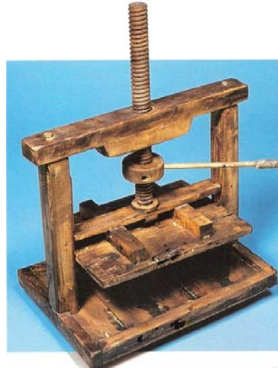
Figure 14: Representation of the oil press operated by an endless screw, and modern reproduction by D. Kriaris [Reference 29]
