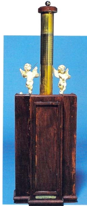
Figure 12: The water clock of Ktesibius and reproduction by D. Kriaris [Reference 29]
