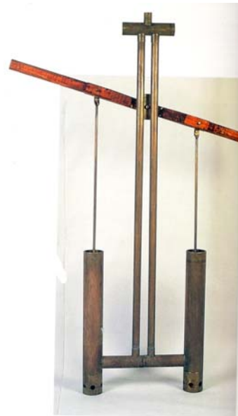
Figure 13: The force pump of Ktesibius and modern reproduction by D. Kriaris [Reference 29]
