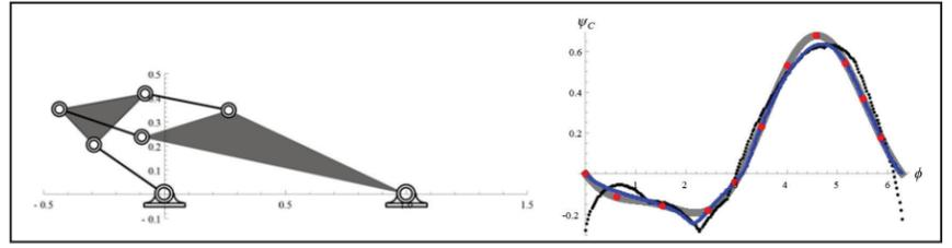
Figure 2. At left, a Stephenson II six-bar linkage designed to transform uniform rotation to a specific joint angle function. At right, comparing the angle of the elbow joint of a bird-wing [3] (black dots), fitted Fourier function (gray), and the function obtained from the synthesized six-bar linkage (blue) passing through 8 of the 11 task points (red dots). Both figures reprinted from [2] with permission.
