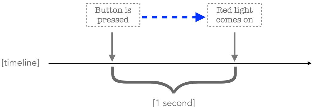
Here the timeline represents the time passed between the two events — 1 second — and the blue arrow represents the direction of causation. (The button pressing causes the light to come on.)
