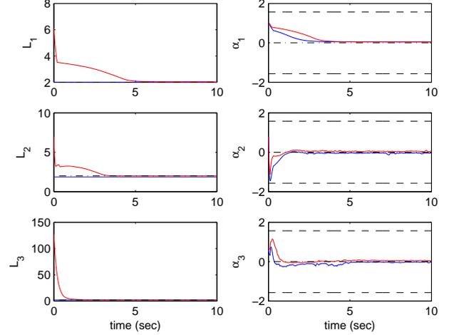
Fig. 4. The maximum and minimum value of separation  $L_j$  and bearing angle  $\alpha_j$  for leader-follower pair,  $j = 1, 2, 3$ .
