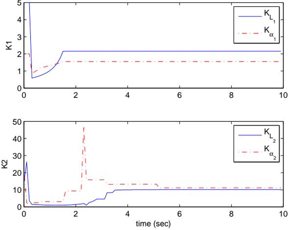
Fig. 5. One sample of switching controller profile for leader-follower pair 1 and 2
