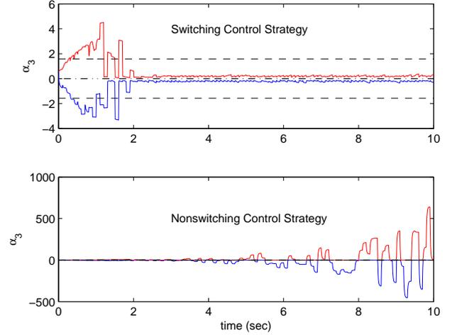
Fig. 7. The maximum and minimum system trajectory for leader-follower pair 3 with switching controller (Top) and non-switching controller pair (Bottom)  $K_{L_3} = 2$  and  $K_{\alpha_3} = 50$
