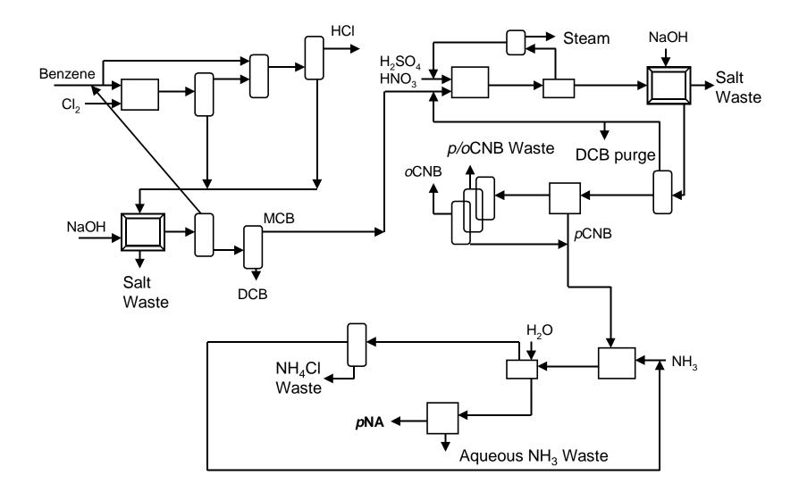
Figure 6. Conventional process for the production of *p*-nitroaniline. The process chemistry is shown in Fig. 5.
