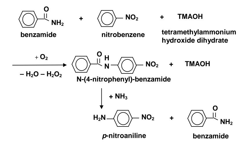
Figure 7. Chemistry for production of *p*-nitroaniline using the new technology.
