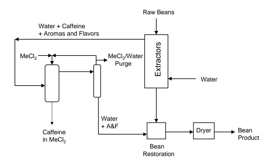
Figure 1. Conventional "water process" for decaffeination of coffee beans.
