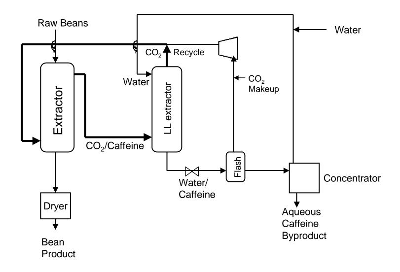
Figure 2. Decaffeination of coffee beans using supercritical CO<sub>2</sub>.
