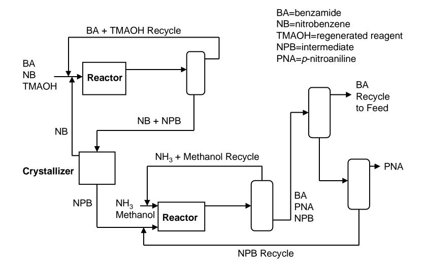
Figure 8. New process for the production of *p*-nitroaniline that uses nucleophilic aromatic substitution and eliminates chlorobenzene as an intermediate. The process chemistry is shown in Fig. 7.
