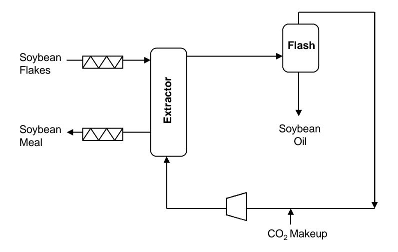
Figure 4. Process for the extraction of soybean oil using supercritical CO<sub>2</sub>.
