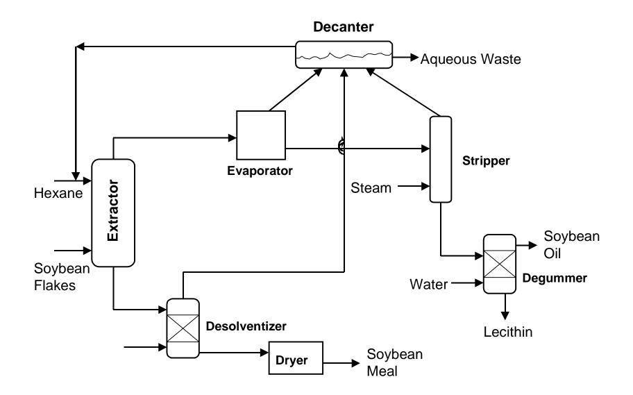
Figure 3. Conventional process for soybean oil extraction using hexane.
