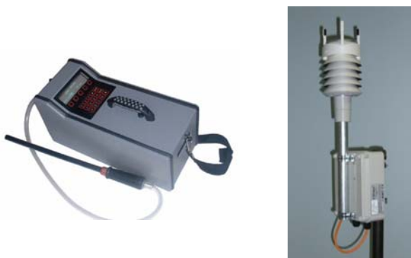
FIGURE 1. InfraRan specific vapor analyzer (left) and WTX510 meteorological sensor wired to I-Node platform.
