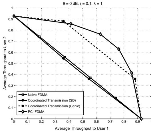
Figure 4: Average Link Throughputs for  $\theta = 0$  dB,  $r = 0.1$ .
