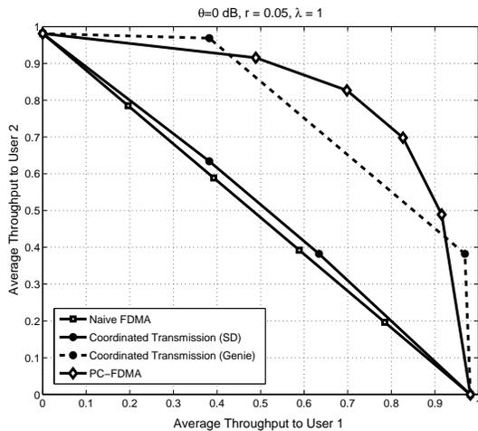
Figure 3: Average Link Throughputs for  $\theta = 0$  dB,  $r = 0.05$ .
