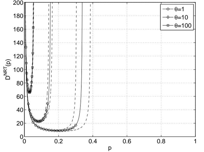
Fig. 3. The local delay for the static NRT case as a function of the channel access probability  $p$  for  $\alpha = 4$  and  $\theta = 1, 10, 100$ . The dashed lines are the upper and lower bounds (25) and (26), respectively.
