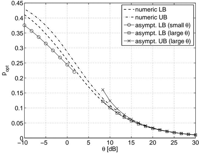
Fig. 5. The optimum transmit probability for the static NNT case as a function of the SIR threshold  $\theta$  for  $\alpha = 4$ . The numeric bounds are obtained by numerically optimizing over  $p$  when the upper and lower bounds from Thm. 3 for  $\kappa^{\text{NNT}}$  are used. The lower and upper bounds for large  $\theta$  are the ones in (39) and (40), respectively. The asymptotic lower bound as  $\theta \rightarrow 0$  is from (42).
