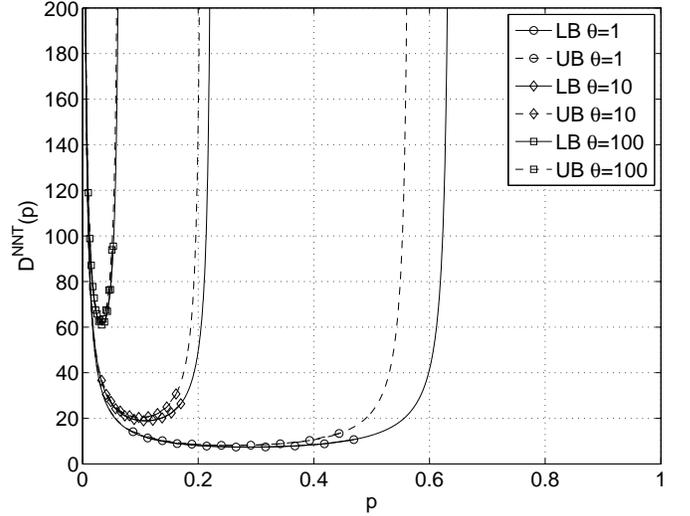
Fig. 4. Bounds on the local delay for the static NNT case as a function of the channel access probability  $p$  for  $\alpha = 4$  and  $\theta = 1, 10, 100$ . The bounds are obtained by inserting the bounds on  $\kappa^{\text{NNT}}$  in Thm. 3 in the delay expression (38).
