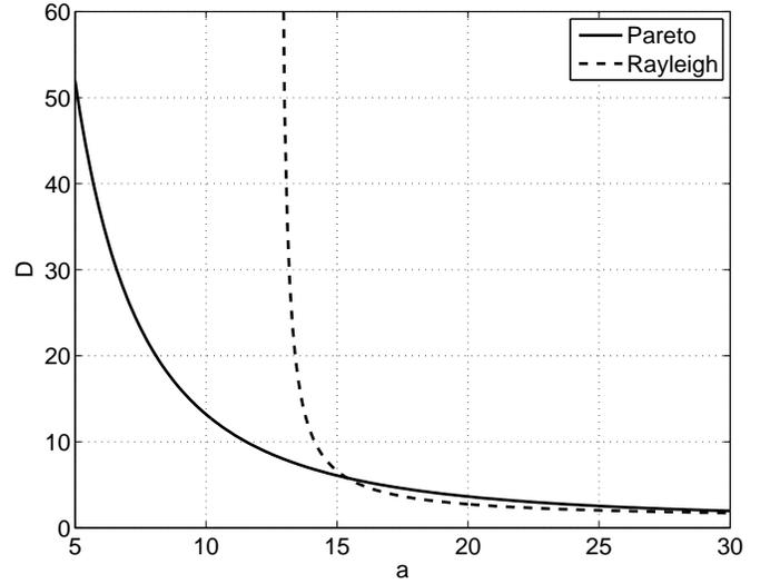
Fig. 9. The mean delay for Rayleigh fading case and Pareto random power control ( $k = 2$ ) for  $b = 0$ ,  $\theta = 10$ ,  $\lambda = 1/4$  (such that the mean link distance  $\mathbb{E}(R) = 1$ ). The phase transition in the Rayleigh case occurs at  $a = \theta/(\lambda\pi) = 40/\pi \approx 12.7$ .
