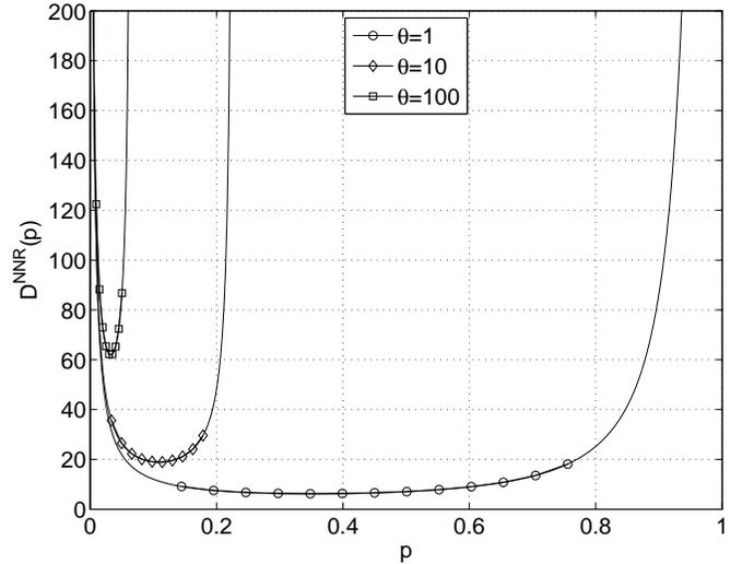
Fig. 7. The local delay for the static NNR case as a function of the channel access probability  $p$  for  $\alpha = 4$  and  $\theta = 1, 10, 100$ . The delay is given in (48).
