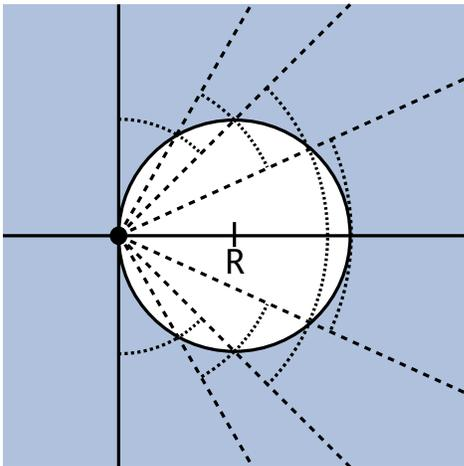
Fig. 11. Illustration for the proof of Thm. 1. The white disk is the interference-free region of nearest-neighbor transmission (NNT). The receiver is located at the origin, and the four sectors (per quadrant) indicate the inner and outer bounds on the disk that are used to obtain analytical bounds on the spatial contention. The angles of the radial beams are  $\pi/6$ ,  $\pi/4$ , and  $\pi/3$ .
