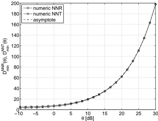
Fig. 6. The minimum local delay for the static NNT and NNR cases as a function of the SIR threshold  $\theta$  for  $\alpha = 4$ . The curves are very close; at small  $\theta$ , the delay for NNT is slightly larger. The asymptote is  $4\gamma/\pi$ , per (41), in both cases. It is quite tight as soon as  $\theta > 1$ .
