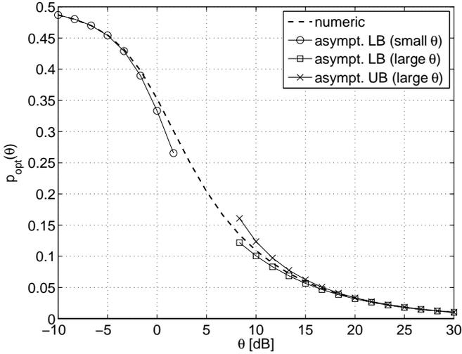
Fig. 8. The optimum transmit probability for the static NNR case as a function of the SIR threshold  $\theta$  for  $\alpha = 4$ . The numeric curve is obtained by numerically optimizing over  $p$ . The lower and upper bounds for large  $\theta$  are the ones in (39) and (40), respectively (same as for the NNT case). The asymptotic lower bound as  $\theta \rightarrow 0$  is from (50).
