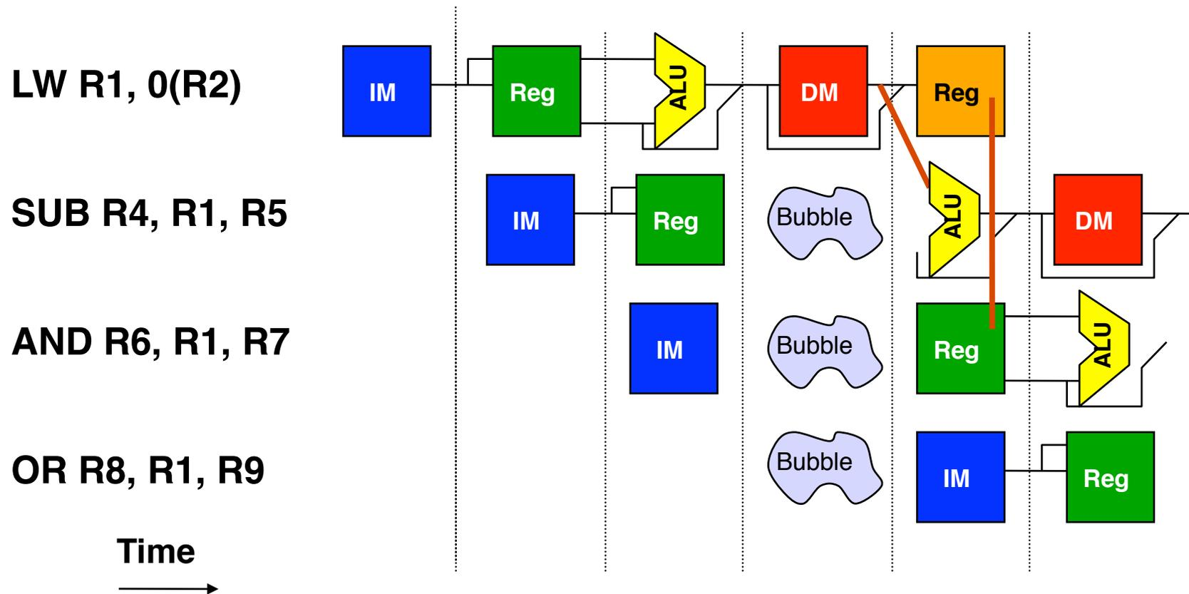
Insertion of bubble causes # of cycles to complete this sequence to grow by 1
