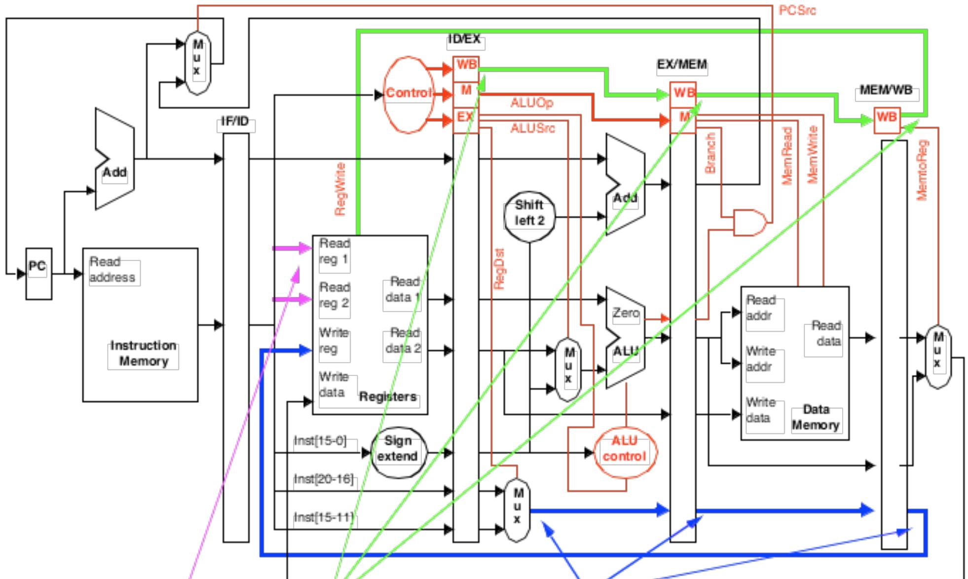
**Hazard if a current register read address = any register write address in pipeline and RegWrite is asserted in that pipeline stage**
