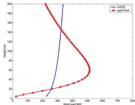
Figure 2. ESWL in ASCE 7 and gust-front wind
