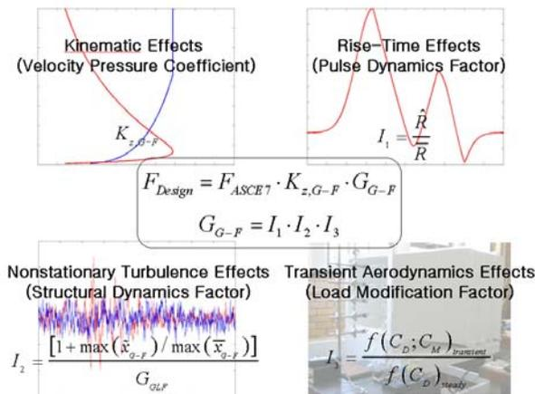
Figure 1. Schematic diagram of gust-front factor and its sub-factors (Kareem et al.<sup>5</sup>)
