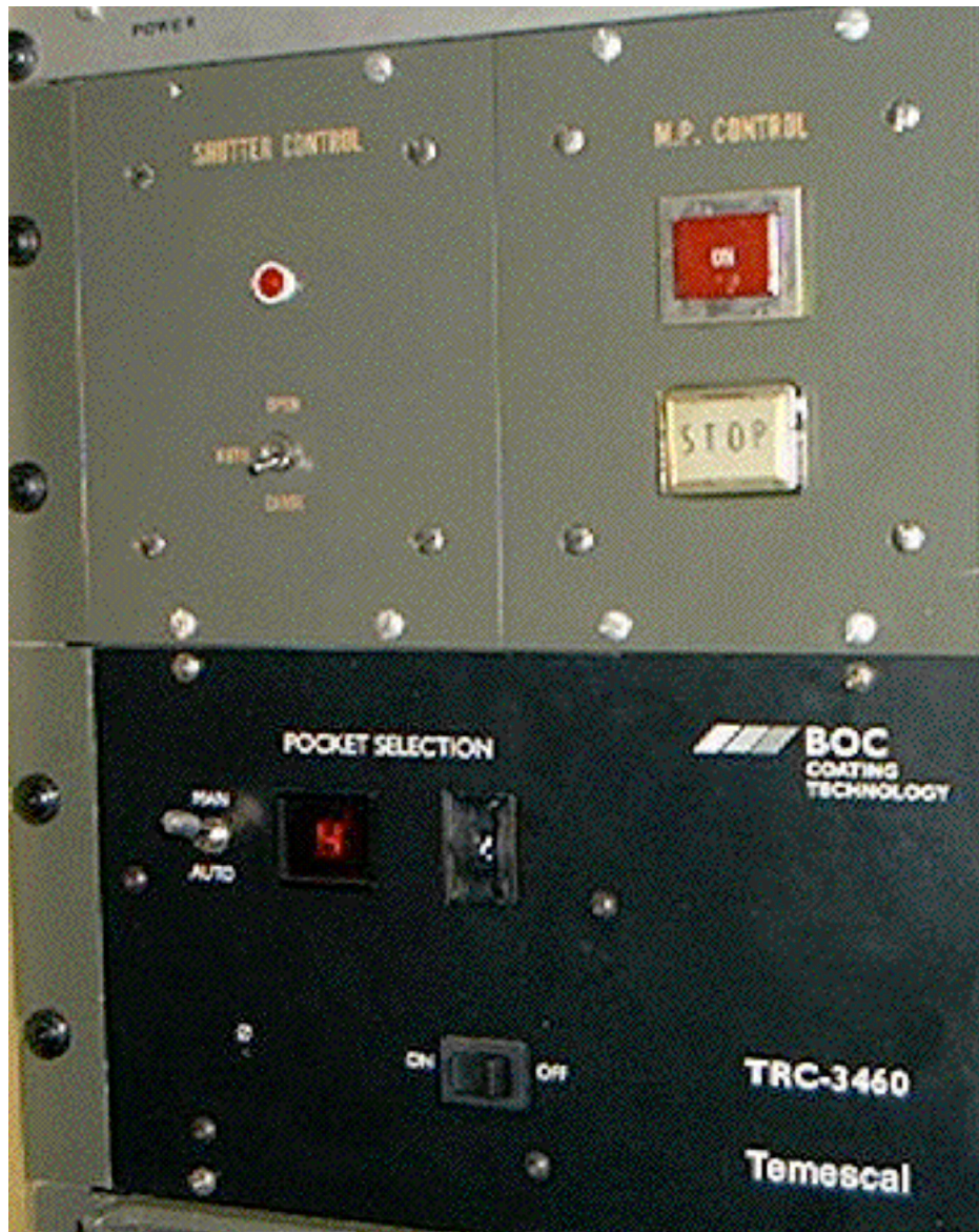
Figure 6: Shutter Control (Top Left), Mechanical pump Control (Top Right), and Pocket Selector (Bottom).
