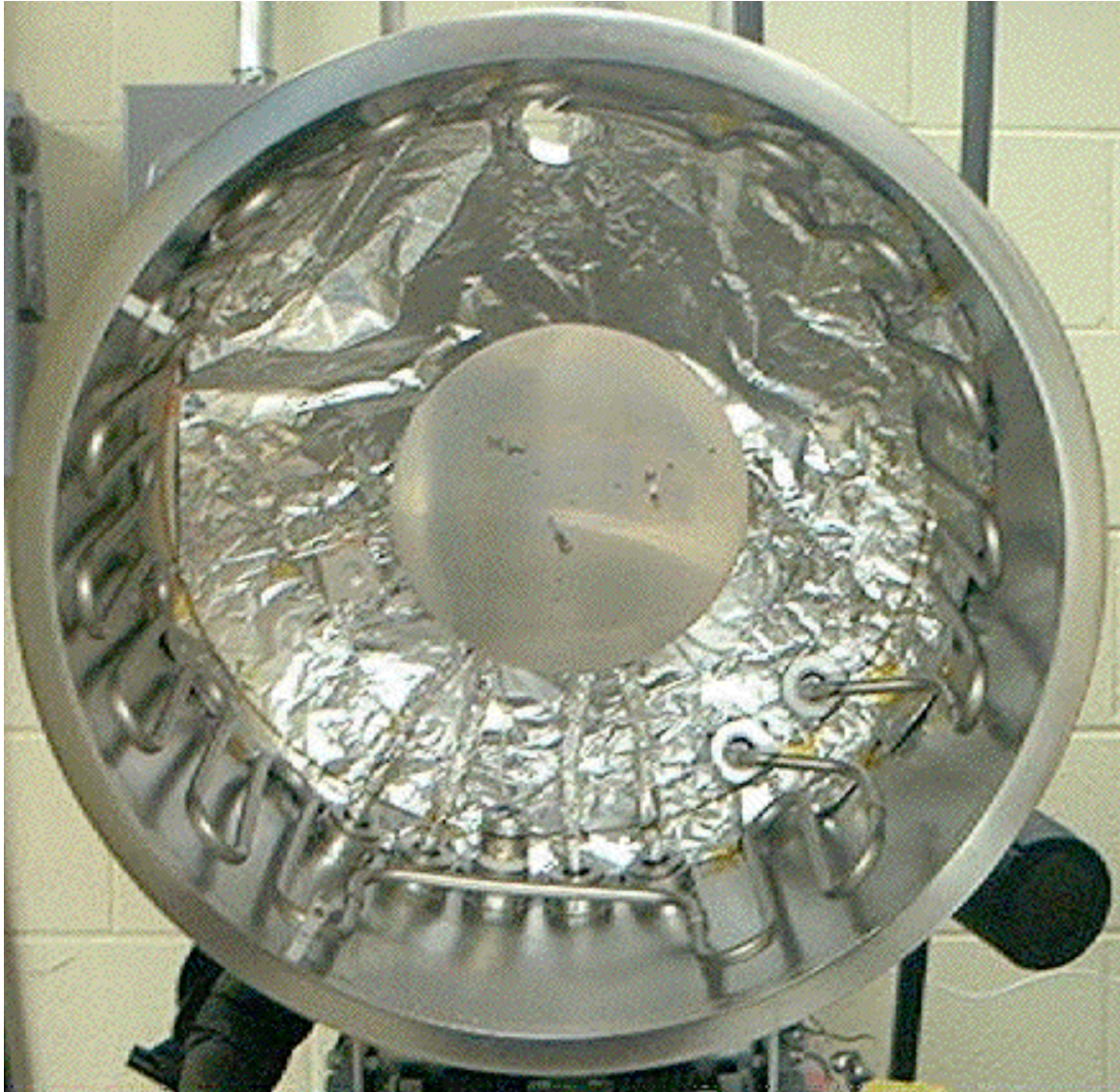
Figure 3: Lid Interior Lid Sample holder in the center and cooling coils on the outer edge of the lid.
