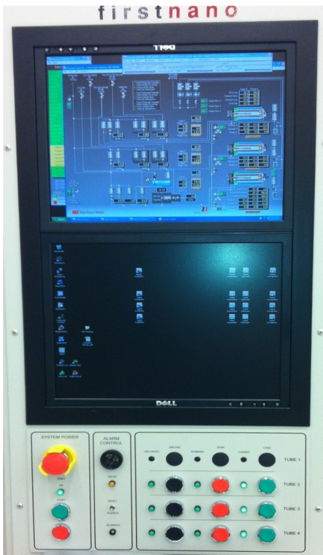
Figure #1: Main LPCVD Controls with monitors on the top and in the middle with loading controls on the bottom.
