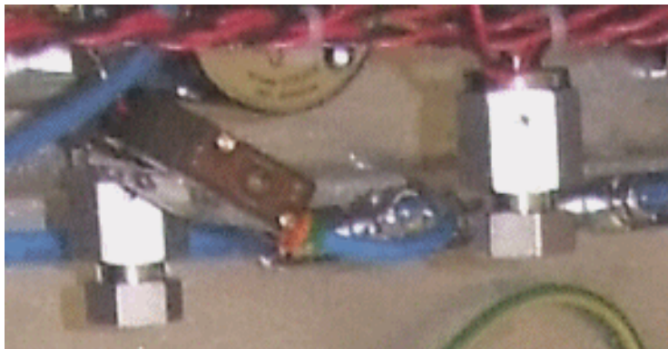
Figure 3-5 VCR connection points for a new ampoule
