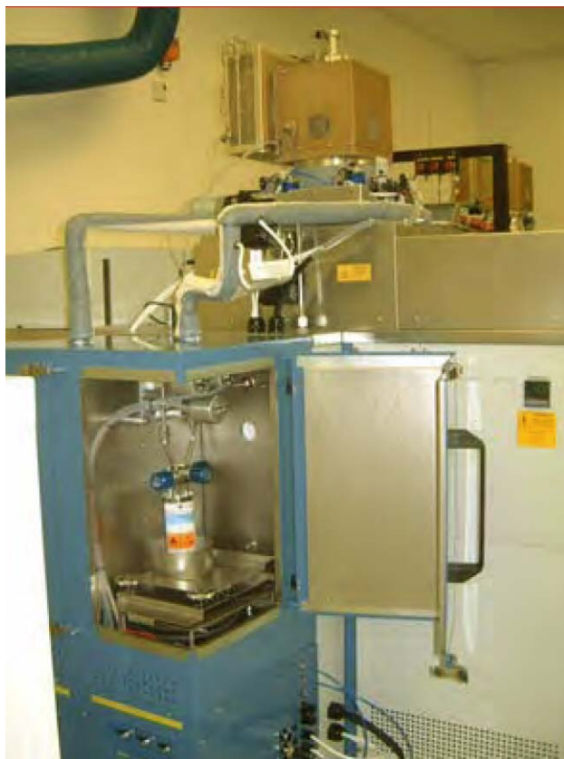
Figure 7-17 Refitting the oven door
