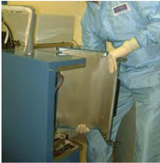
Figure 7-10 Removing the precursor module door
