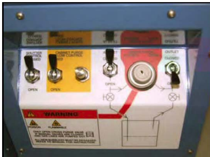
Figure 5-43 PDM controls set for vapour-draw mode
