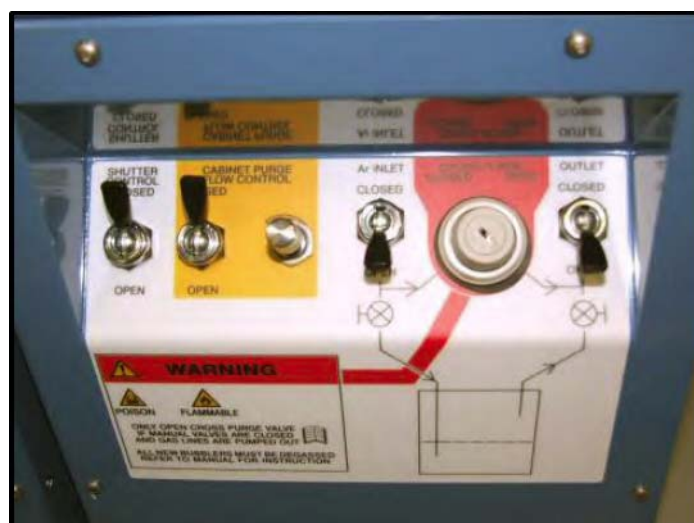
Figure 5-41 PDM controls set for bubbler mode
