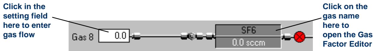
Figure 4-12 Example of gas line in gas mimic
