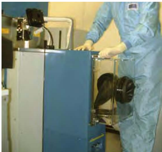
Figure 7-11 Fitting the glove box
