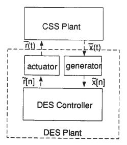
Figure 1: Hybrid Control System Block Diagram
