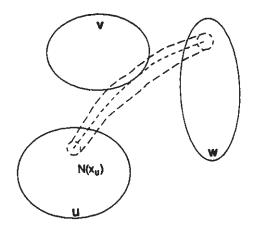
Figure 2: Example of a hybrid system whose logical transition is unstable
