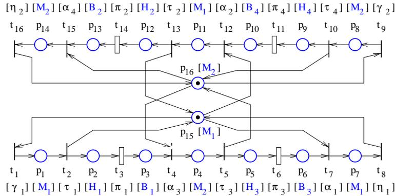
Figure 3: Petri net model of the system.
