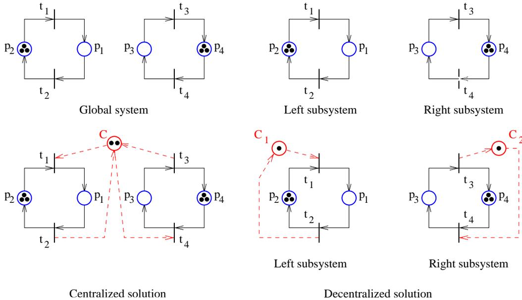
**Figure 1:** Decentralized control example.
