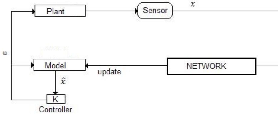
Fig. 1. Representation of a Model-Based Networked Control System.
