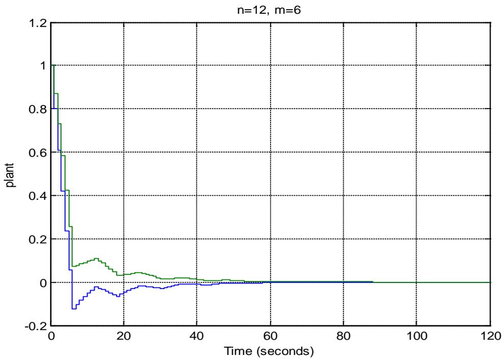
Fig. 13. Response of the plant for  $n=12$  and a)  $m=1$  (unstable system) and b)  $m=6$  (stable system).
