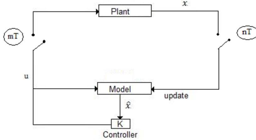
Fig. 7. Model-Based Networked Control System with communication network between sensor-controller and controller-actuator (plant).
