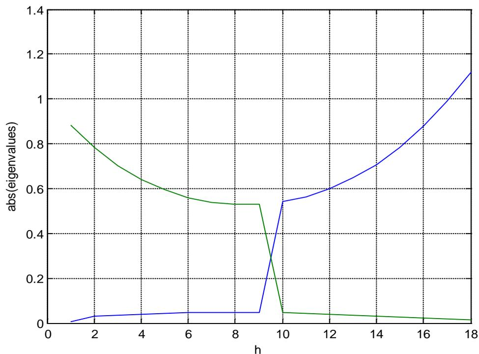
Fig. 3. Absolute value of the eigenvalues of (III.5), showing the values of  $h$  for which the system remains stable.
