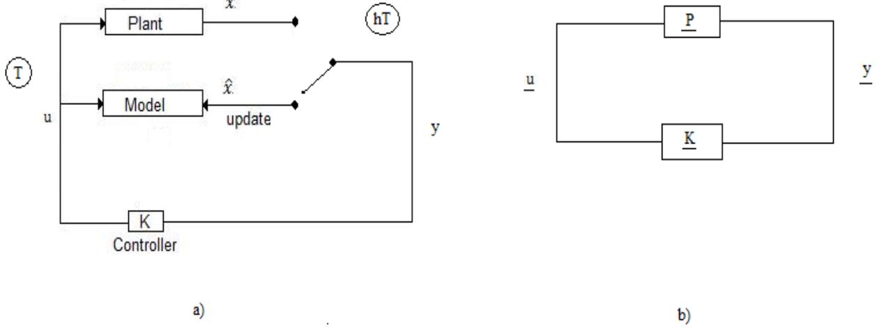
Fig. 2. Equivalent systems to a MB-NCS. a) Linear time-varying system. b) Lifted system.
