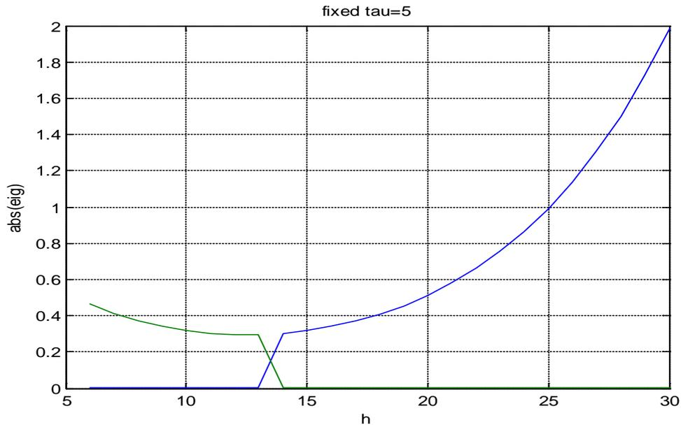
Fig. 5. Absolute value of the eigenvalues of (III.9), showing the values of  $h$  for which the system remains stable.
