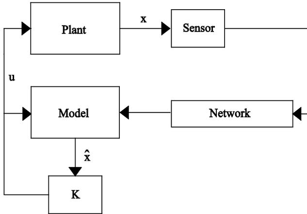
Fig. 1. Representation of a Model-Based Networked Control System.
