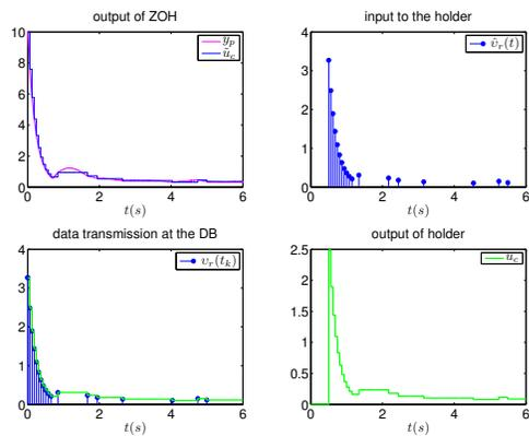
Fig. 5: simulation result of example 1 with constant network induced delay: signal transmission process from  $y_p$  to  $u_c$
