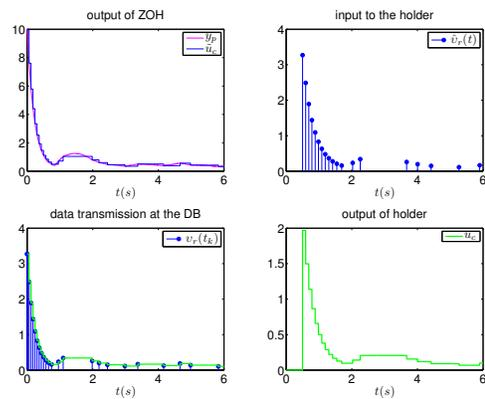
Fig. 7: simulation result of example 1 with time-varying network induced delay: signal transmission process from  $y_p$  to  $u_c$
