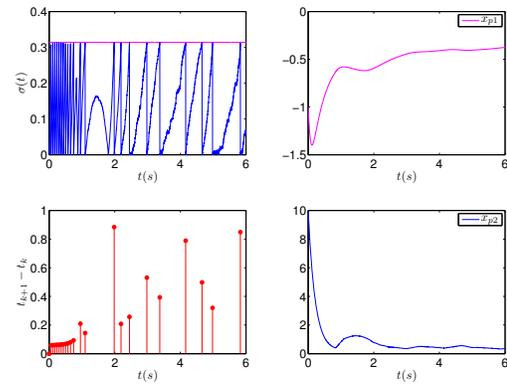
Fig. 6: simulation result of example 1 with time-varying network induced delay: triggering process and state evolution
