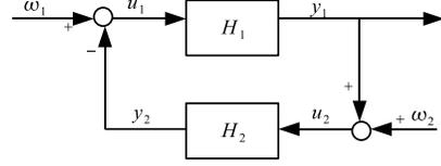
Fig. 1: Feedback Interconnection of Two IF-OFP Systems
