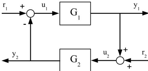
Fig. 1. The negative feedback interconnection of two systems.
