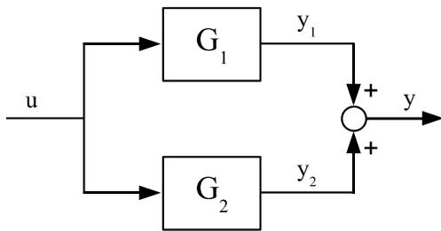
Fig. 2. The parallel interconnection of two systems.
