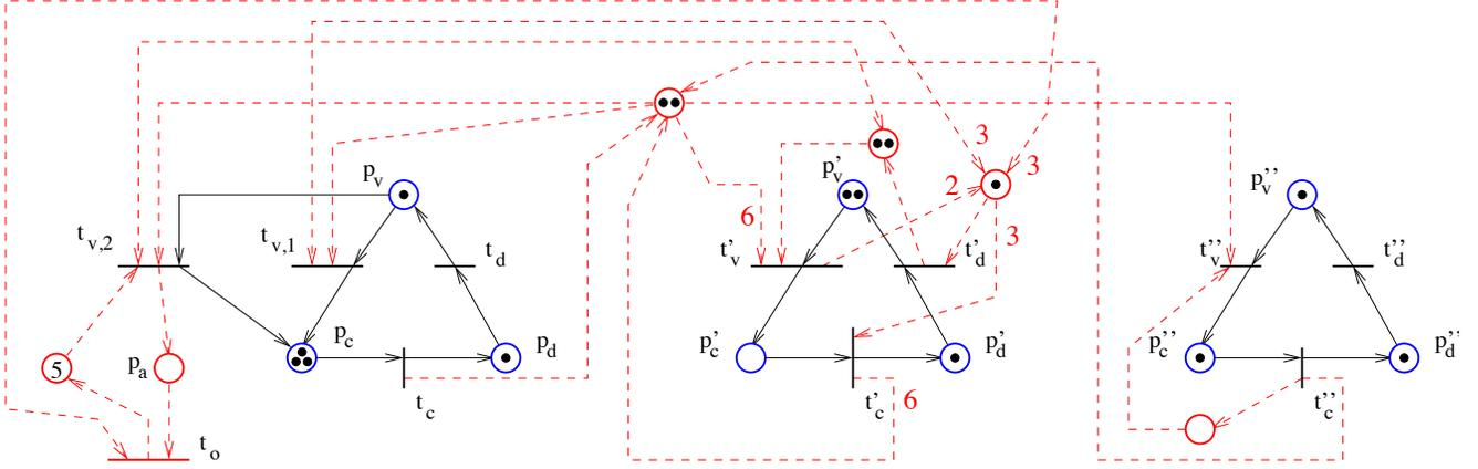
Fig. 4. Supervision in the reader, deleter, and inserter example. A bidirectional arrow between a place  $p$  and a transition  $t$  represents a pair of arcs  $(p, t)$  and  $(t, p)$  of equal weight. A number inside of a place indicates the number of tokens.
