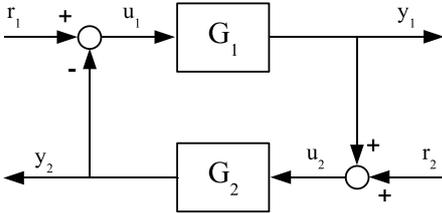
**Bild 1:** The feedback interconnection of two systems  $G_1$  and  $G_2$ .
