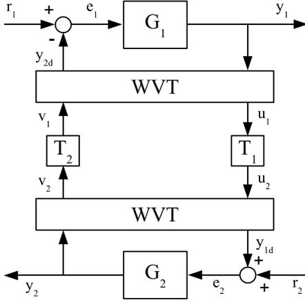
**Bild 3:** The network control structure for passive plants makes use of the wave variable transformation (WVT blocks) on either side of the network. The blocks  $T_1$  and  $T_2$  are the time delays in the network.
