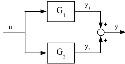
**Bild 2:** The parallel interconnection of two systems.
