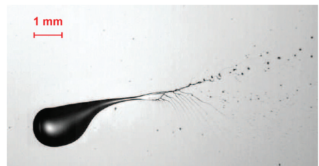
Figure 13. Ramified break-up mode of the jet emanating from the parent drop, m = 2 .
