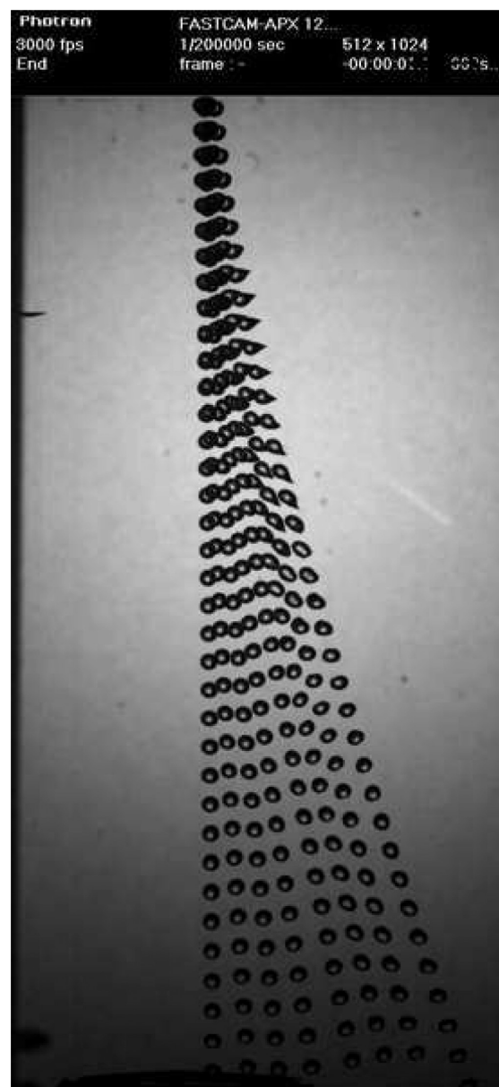
Figure 2. Parent drop trajectories at various applied voltage differences (0–50 kV). The distance between the tip of the corona needle and the grounded electrode was 8 cm. The initial drop diameter was 2.21 mm.
