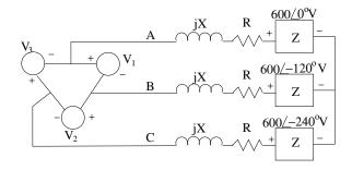
4. Here we have a generic, balanced 3-phase system. Don't be confused by the somewhat different look of this graph; it's a Δ-connected source driving a Y-connected load, so V<sub>1</sub>, etc would be the usual Δ voltages. The common load impedance is Z = 30∠30°Ω and line impedances are R = 1Ω and X = 2Ω.
