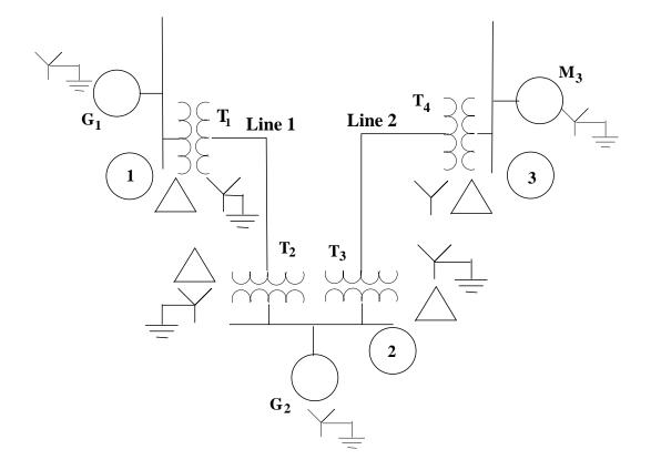
(a) (10 pts.) Find the matrix  $\mathbf{Y}_{bus}$  for power flow computations. (b) (10 pts.) Find the system's  $\mathbf{Y}_{bus1}$  appropriate for the positive sequence component in fault analysis. (c) (15 pts.) Suppose we have the following bus impedance matrices for the system (these are NOT correct for the parameters given at the beginning of the problem):
