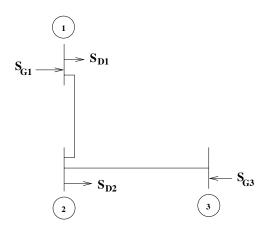
(a) (10 pts.) Find the bus admittance matrix which will be appropriate for solving power flow for the system.
