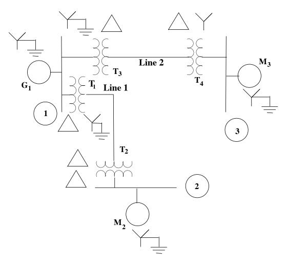
(a) (10 pts.) Find and sketch the equivalent circuit in pu for the zero sequence component for analysis of this system under  $S_{base} = 100$ MVA, and  $V_{base} = 13.8$ kV at generator 1. (b)(10 pts.) Find the value of the first element (1,1) in the  $Z_{bus0}$  matrix for symmetric components analysis.
