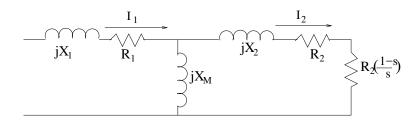
(a) (13 pts.) Find the number of poles in the windings and, at rated load, the rotor slip, the rotor electrical frequency, and the power converted from electrical to mechanical,  $P_{conv}$
