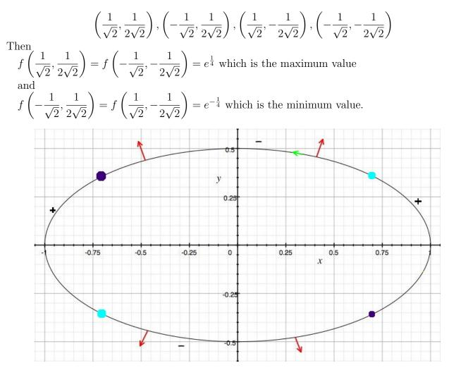
The light blue dots are the approximate locations of the maxima and the purple dots are the approximate locations of the minima. You can pick out the intervals where f is increasing and where it is decreasing as you move along the curve in the preferred direction and note that it is consistent with the calculations of H above.
