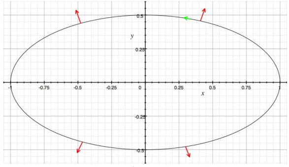
The red vectors point in the direction of the gradient  $\nabla g$  and the green arrow indicates the preferred direction along the constraint curve.
