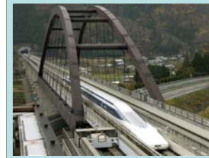
Manned MLX01-901 train at the Yamanashi Maglev Test Line in Japan. This train have reached a speed of 360 mph and sustained a two-train crossing test at a relative speed of 637 mph.
