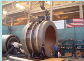
36.5 MW ship propulsion motor manufactured by American Superconductor.
