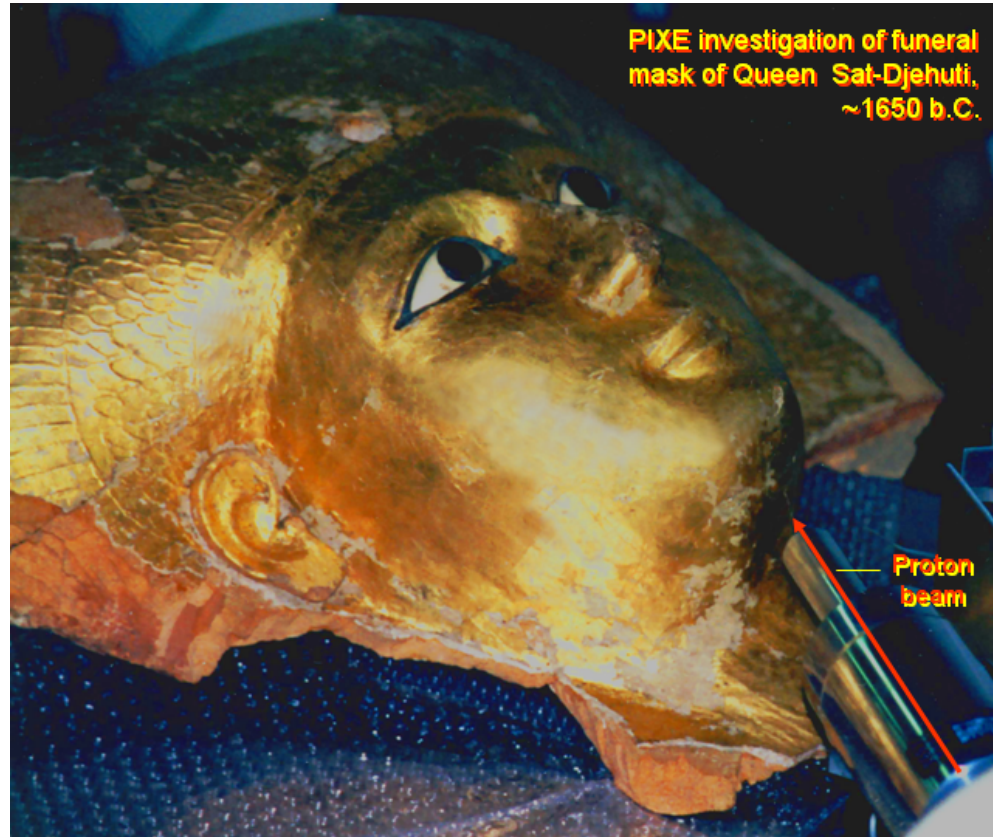
Figure 71: PIXE investigation of the gold plated funeral mask of Queen Sat Djehuti at the HMI Berlin.
