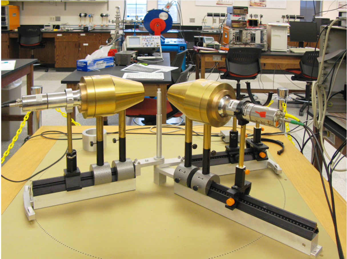
Figure 47: Photo of the set-up for the measurement of gamma-angular distributions with two NaI-detectors. One detector is fixed in its position, the other is moveable by increments of exactly 1^\circ . The angular scale was produced by drilling holes in an aluminum plate on top of the experimental table.
