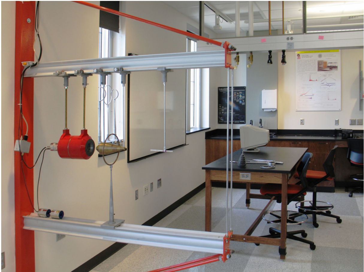
Figure 37: Set-up of the the Compton experiment with ring geometry for cross section determination. Note the considerable distances for all structural elements which contribute to background.
