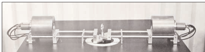
Fig. 19.8 The Model 306 Angular Correlation Table Originally Manufactured by Metrix.
