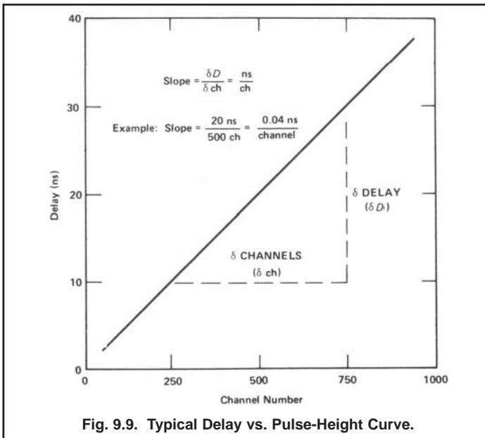
Fig. 9.9. Typical Delay vs. Pulse-Height Curve.
