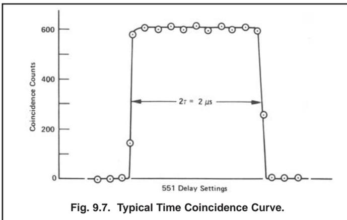
Fig. 9.7. Typical Time Coincidence Curve.
