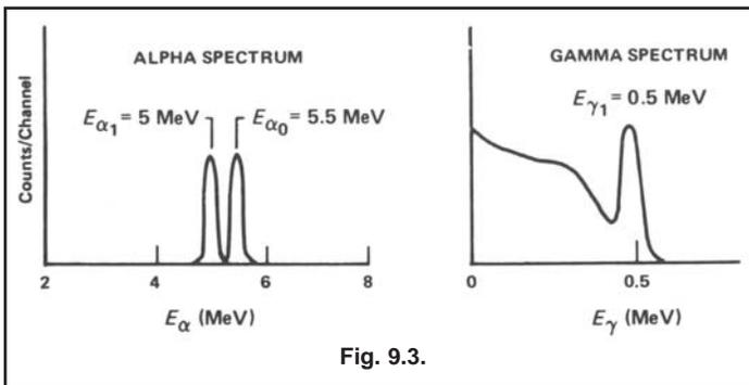
If the electronics are set up with a surface barrier detector to look at the alphas and with a NaI(Tl) detector to look at the gammas, it will be observed that there are no gammas in coincidence with  $\alpha_0$ .
