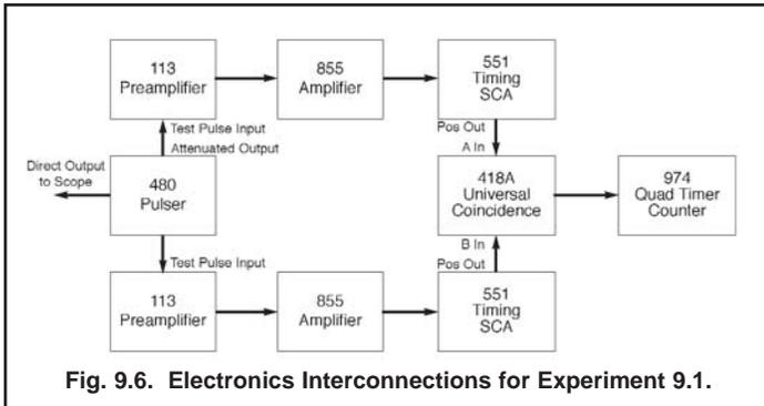
Fig. 9.6. Electronics Interconnections for Experiment 9.1.
