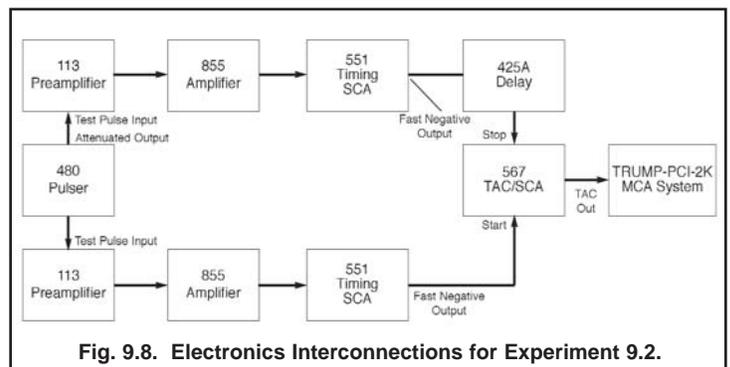
Fig. 9.8. Electronics Interconnections for Experiment 9.2.
